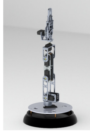
Figure 3. Dagu robotic arm with 6 degrees of freedom used in our experiment.
