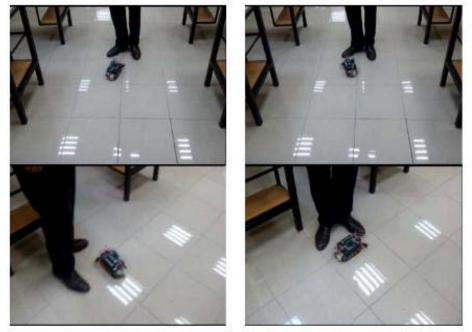
Figure 11: Photos from the video sequence in our Lab of the closely spaced obstacles experiment. Repulsive forces obliged the robot to turn away when it in front of our colleague
