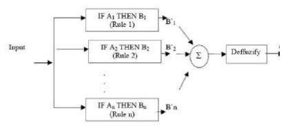
Figure 7: Fuzzy controller used in our method for robot collision avoidance
