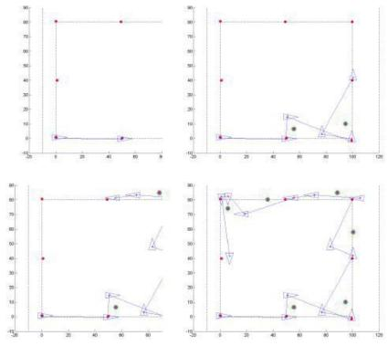
Figure 9: Robot navigation with avoidance of dynamical obstacles (humans) represented with bold discs surrounded with a green circle
