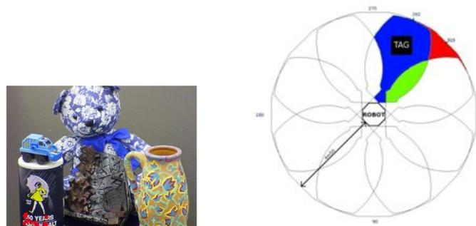
Figure 2: Reception field of one antenna (left). Reception field of eight antennas monted on a circular robot (right)
